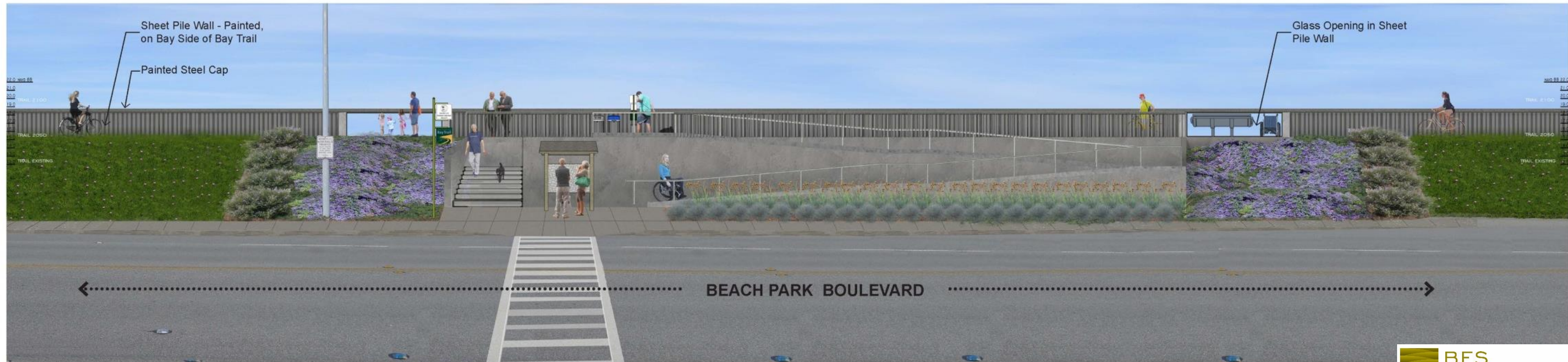
Typical View of Access along Beachpark Boulevard Levee Wall - Grey Sheetpile Wall with Steel Cap and 10'-0" Wide Glass Openings at Access Points
