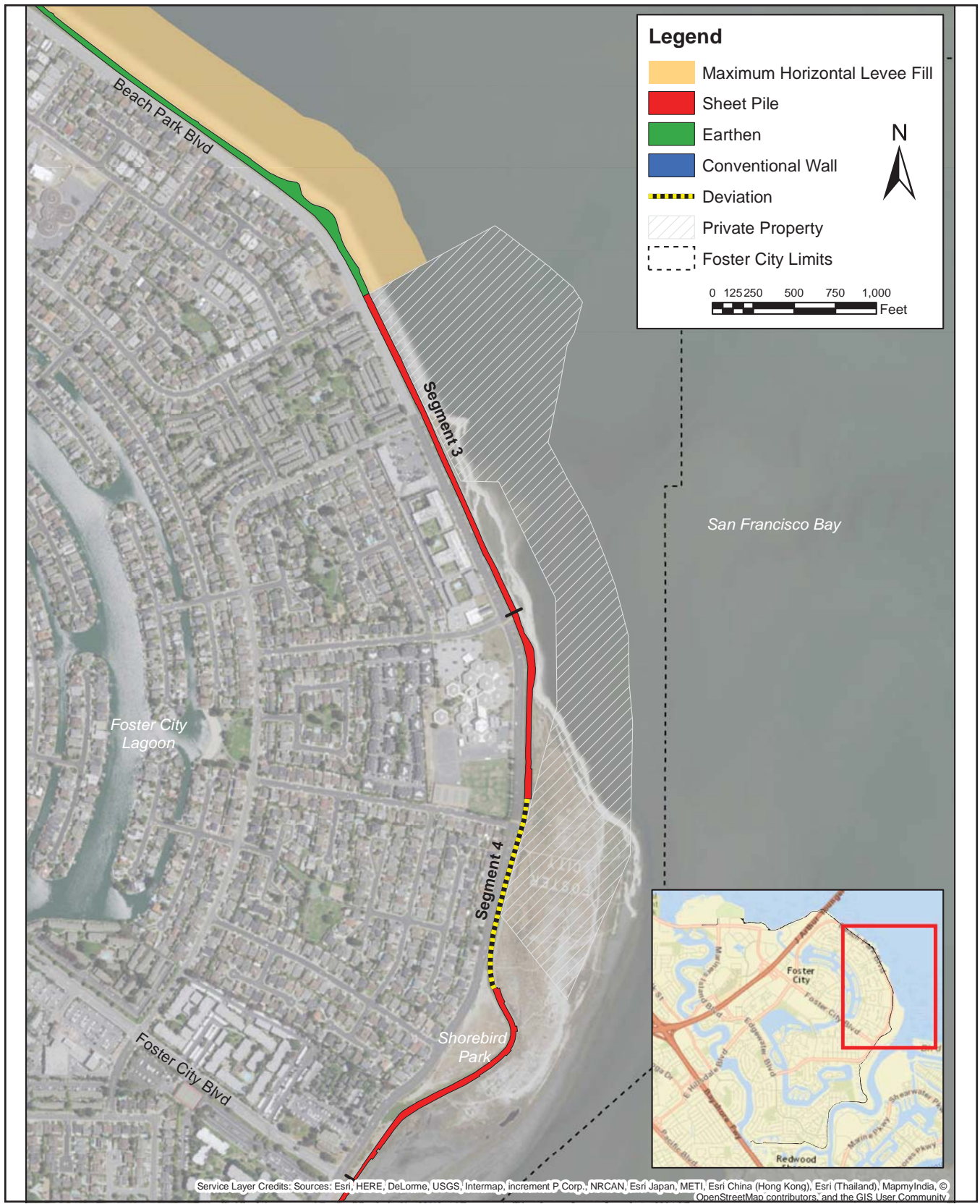
Figure VI-2 Foster City Levee Protection Planning and Improvements Project EIR Horizontal Levee 2050 Alternative Close Up
