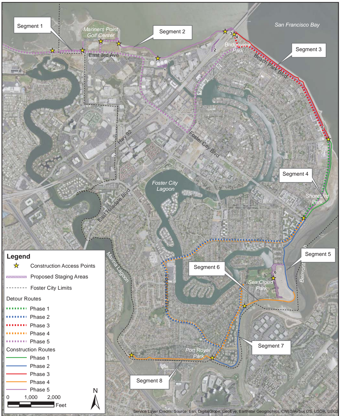
Figure III-16 Foster City Levee Protection Planning and Improvements Project EIR Construction Phasing (2100 Sea Level Rise Scenario)
