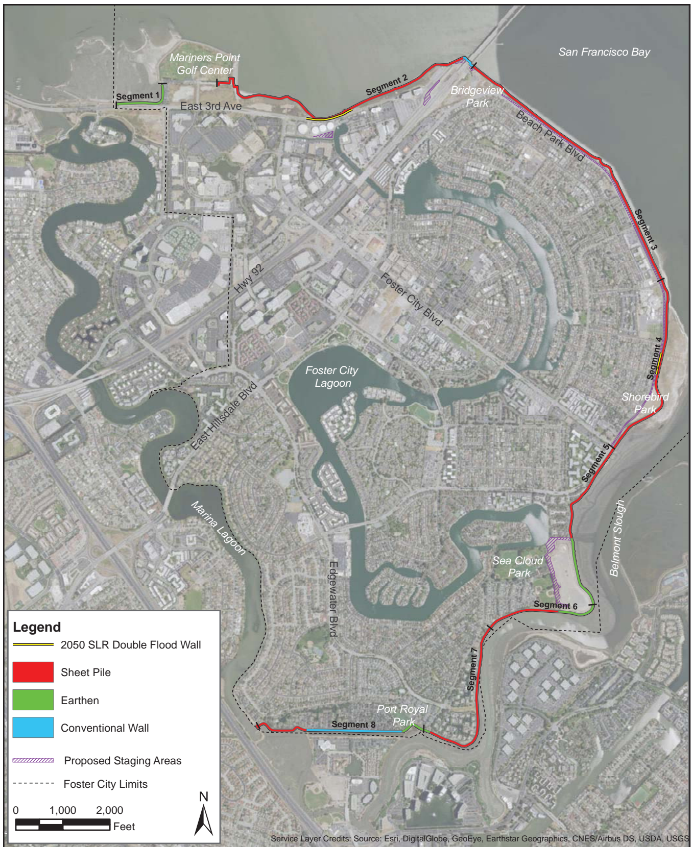
Figure III-3 Foster City Levee Protection Planning and Improvements Project EIR Levee Improvement Type (2050 Sea Level Rise Scenario)
