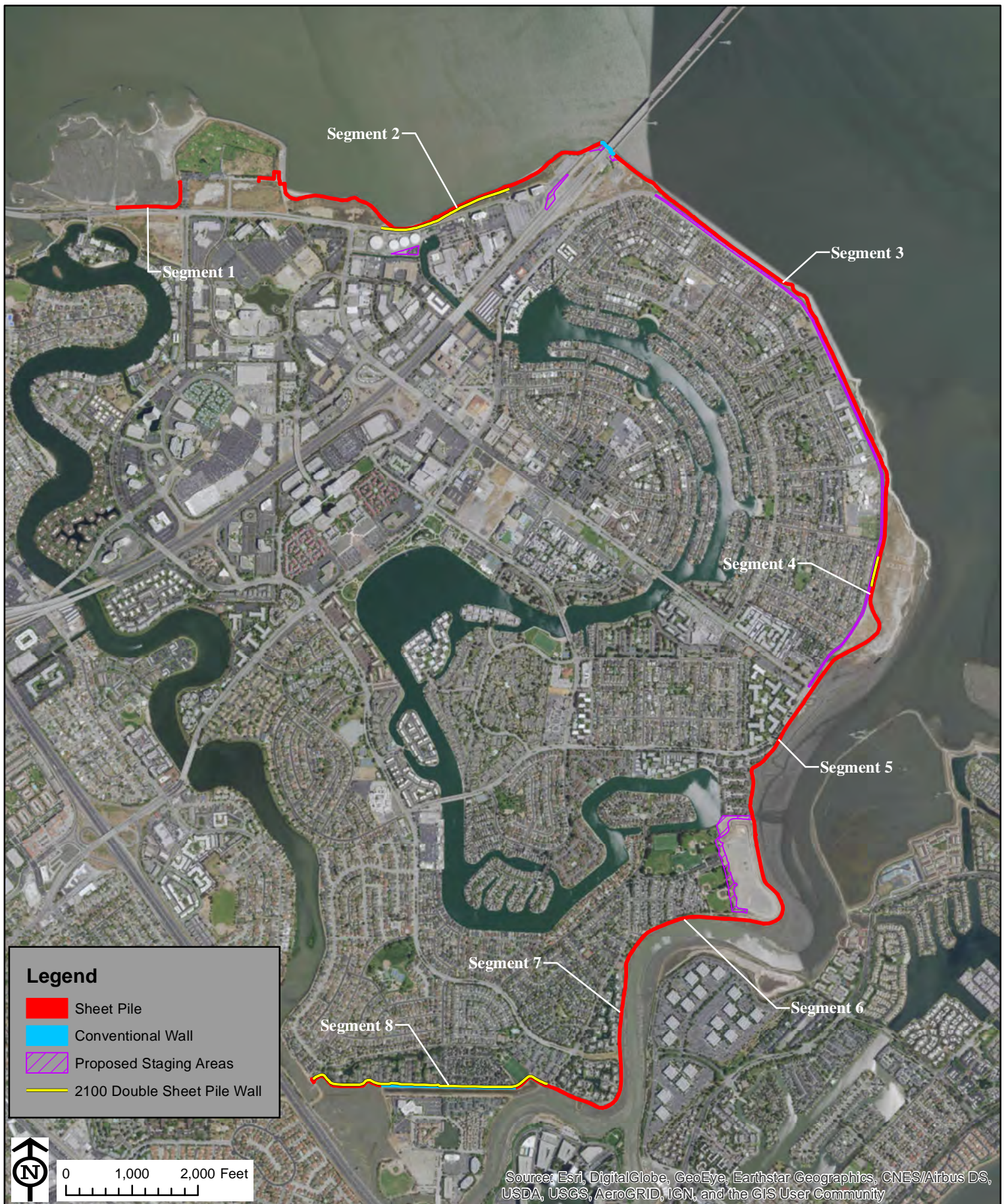
Figure 3. Foster City Levee Protection Planning and Improvement Project Levee Improvement Type for the 2100 Sea Level Rise Scenario
