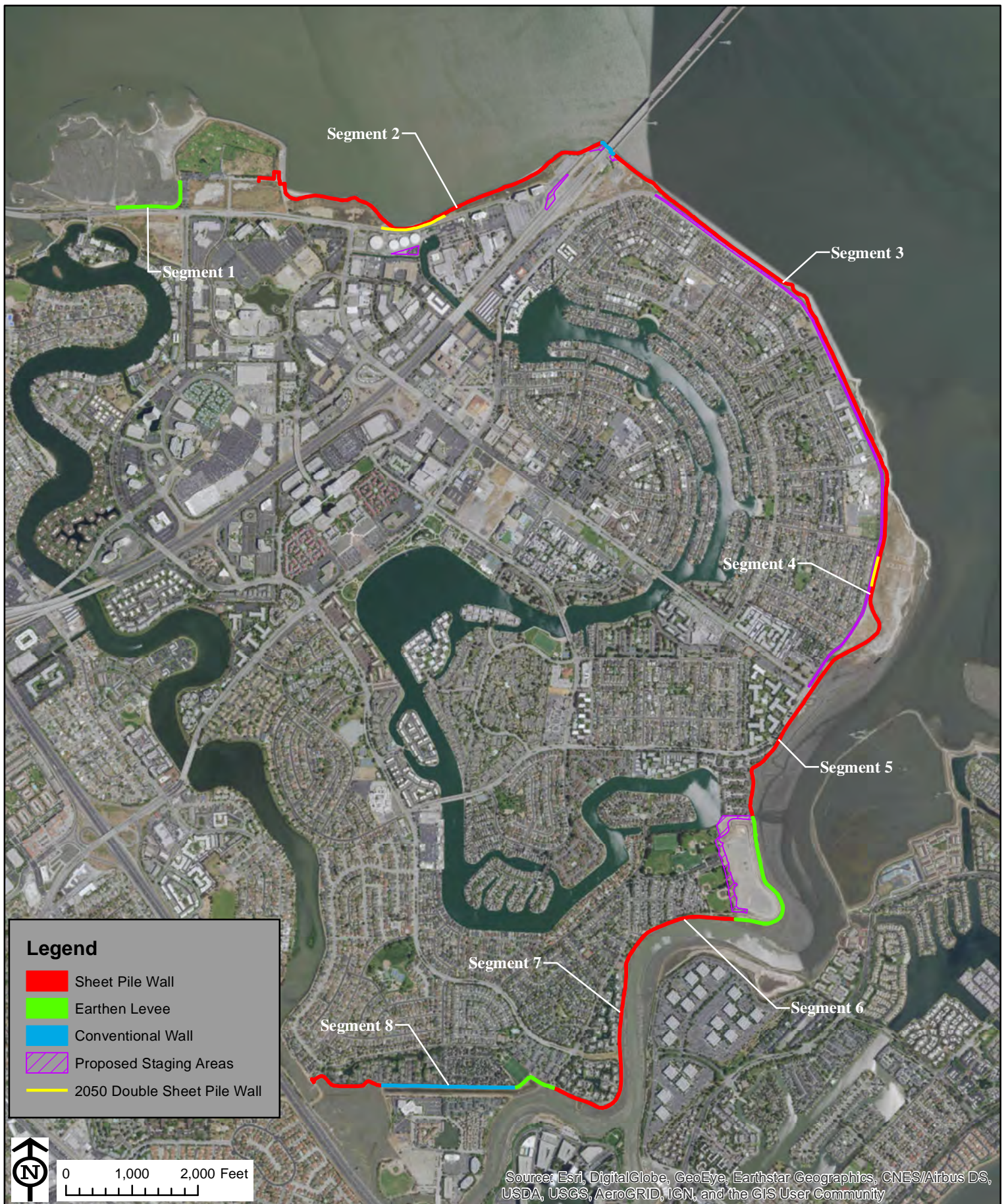
Figure 2. Foster City Levee Protection Planning and Improvement Project Levee Improvement Type for the 2050 Sea Level Rise Scenario
